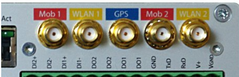
Fig. 4.2: Antenna connectors SMA
