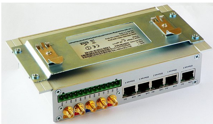
Fig. 4.9: MG102i with DIN rail bracket
