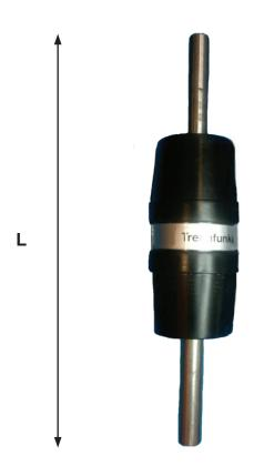
SG closed spark gap can handle lightning discharge currents of 100 kA (8/20 µs). Connection 2 x A2 M10.
