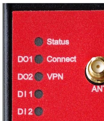
*Fig. 4.6: Indication LEDs*
